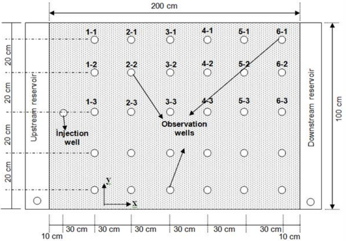
Figure 1. Plan view of the experimental set-up with location and number of the wells
