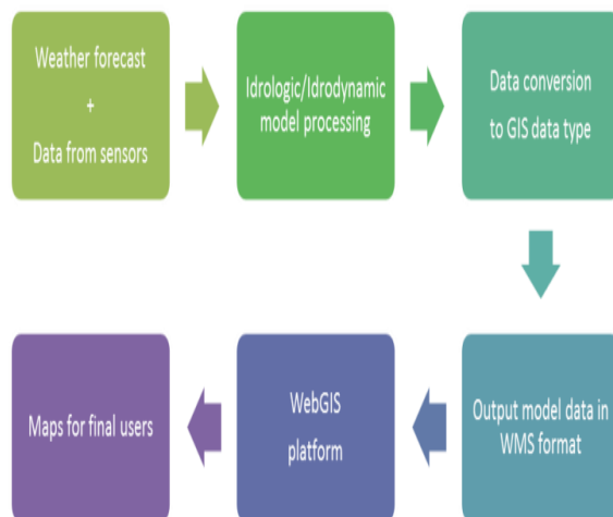
Figure 4. Information flow as it will be implemented in the webGIS tool that will be the result of Smart Water project.
