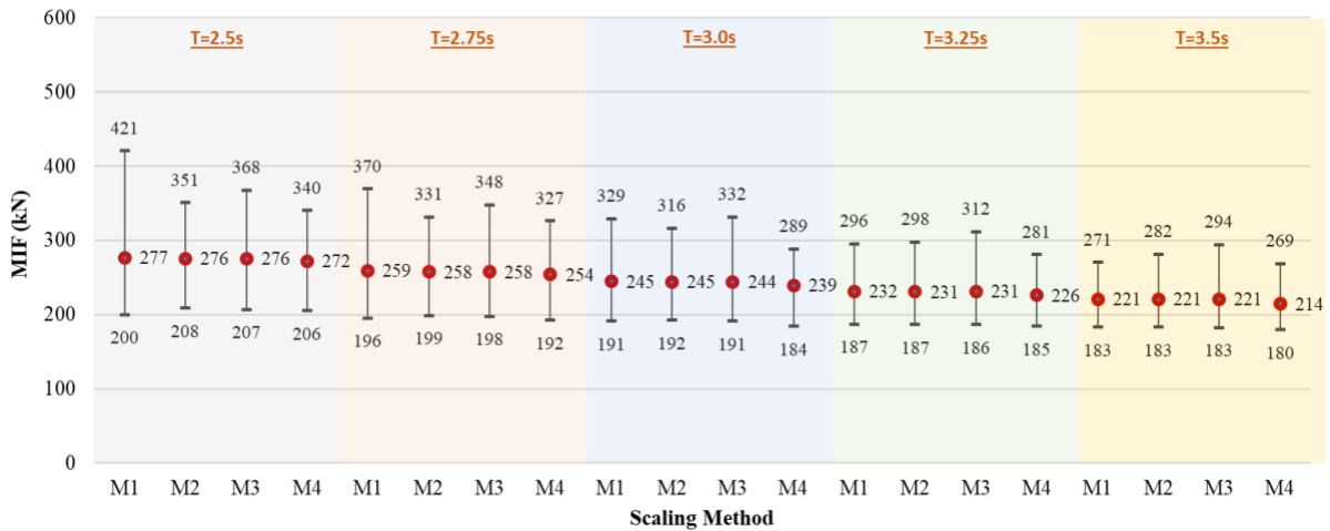
Figure 4. Variation of MIF with period and scaling methods (Q/W=0.105)
