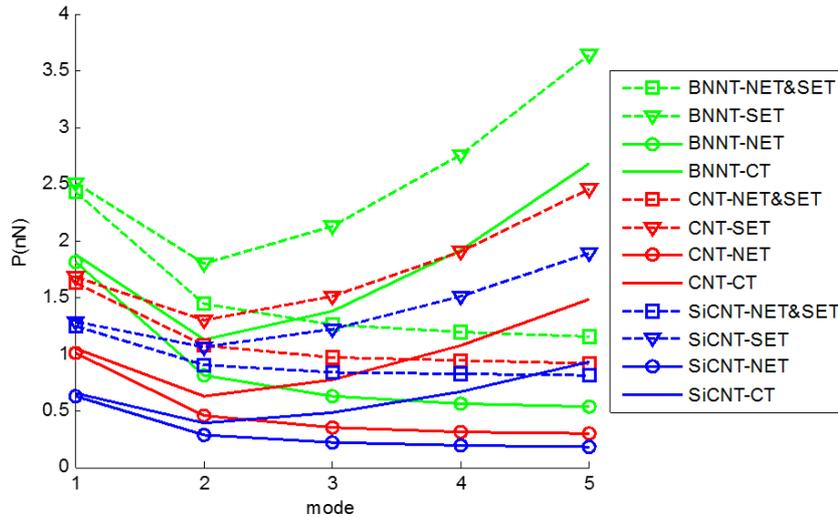
Fig. 5. Buckling loads for different mode numbers
