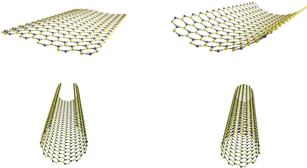
Fig. 1. Obtaining nanotubes
