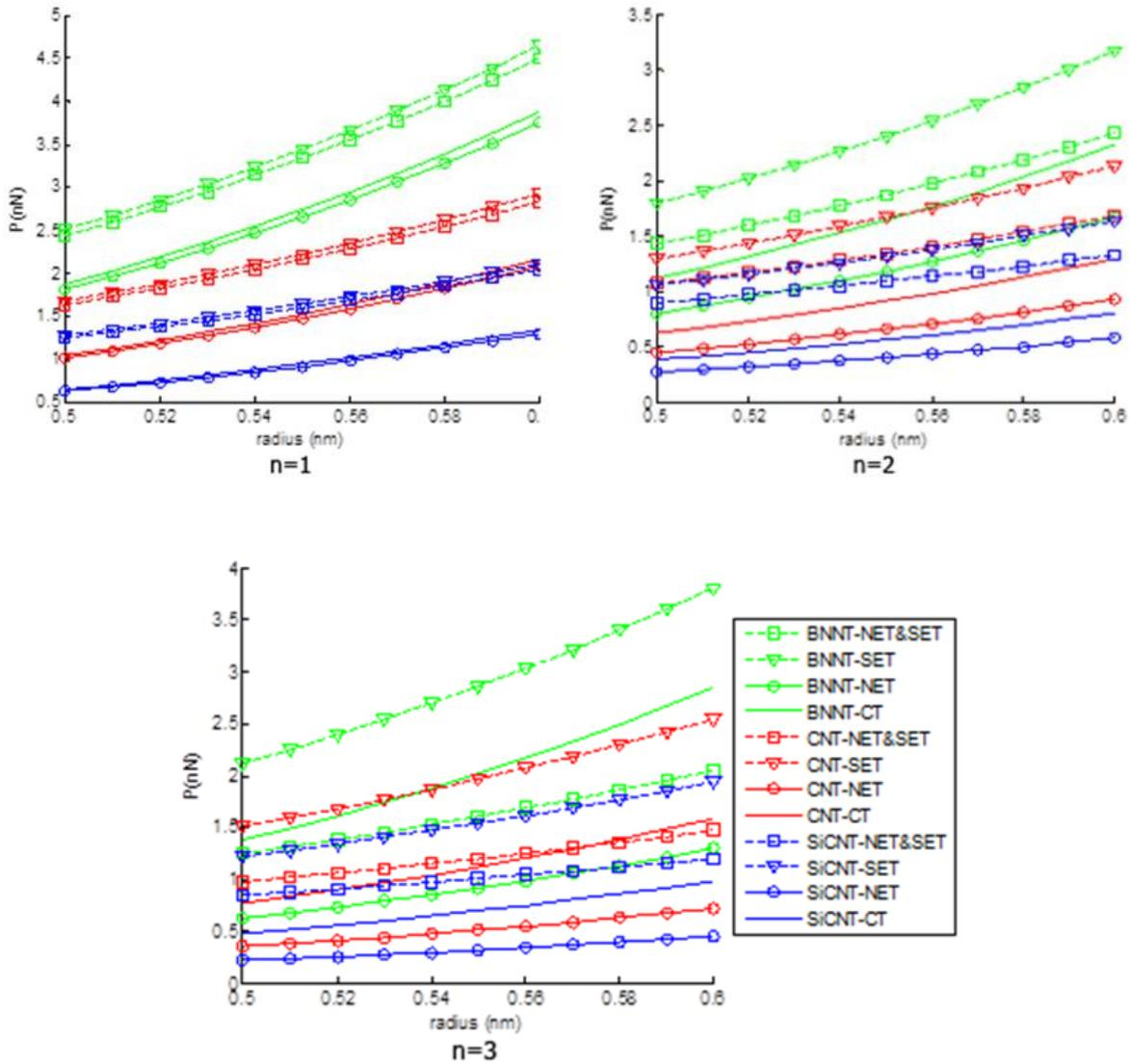
Fig. 4. Buckling loads of nanotubes for various radius
