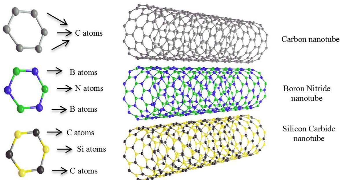
Fig. 3. The structure of CNT, BNNT, and SiCNT
