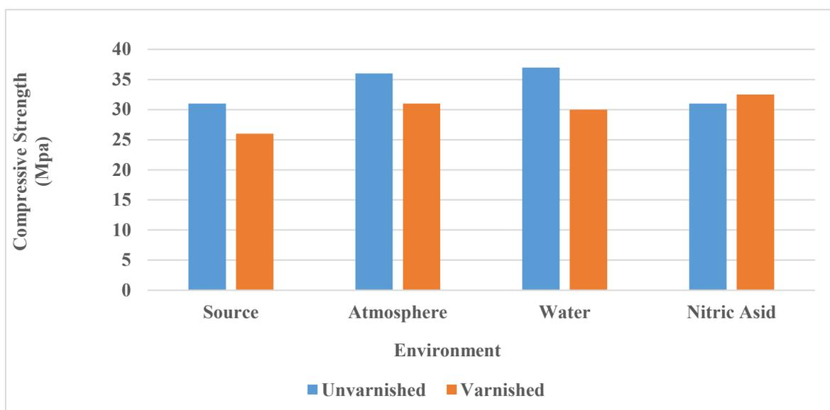
Figure 2. Compressive Strength of samples
