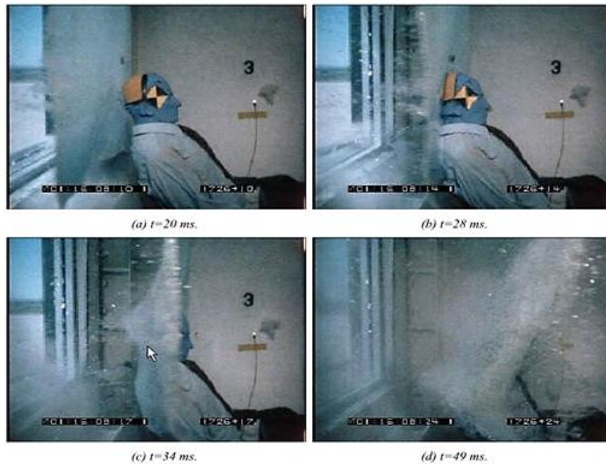
Figure 12. Response of test dummies exposed to blast impact of glass [12]
