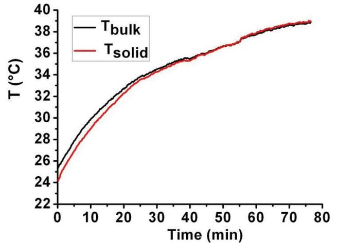
Figure 6. Evolution of water and solid temperatures versus time with two transducers in operation without heating.
