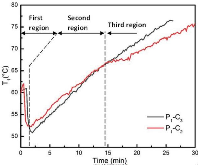
Figure 7. Evolution of the temperature  $T_1$  versus time for C2 and C3 configurations.
