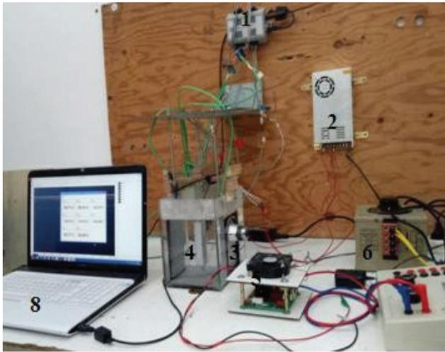
**Figure 2.** Picture of the experimental set-up. 1- Data acquisition, 2- DC power supply, 3- 40 KHz piezoelectric transducers, 4- Water tank, 5- Ultrasonic generator, 6- Voltage variator, 7- Wattmeter, 8- PC.
