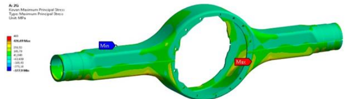
Figure 9. FEA stress results display for 2G loading, max. principal stress
