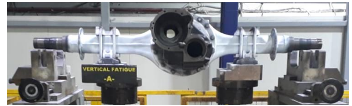
Figure 11. Test set-up front view of an axle housing
