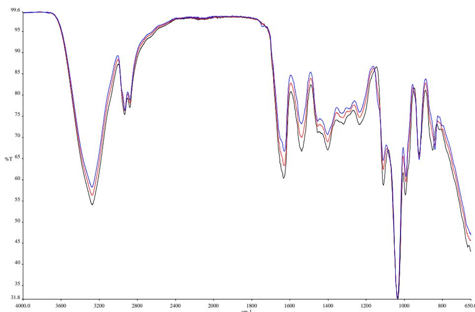
Figure 2. Fourier Transform Infrared (FTIR) spectra of films: WPI (black line), C-WPI (red line), A-WPI (blue line).
