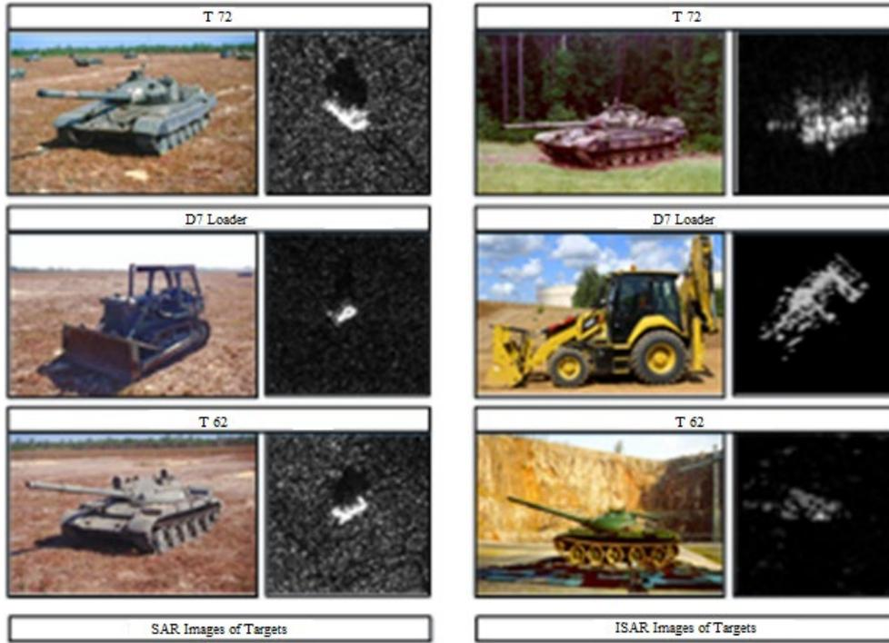
**Figure 1.** Targets and their sample radar images used in the proposed machine-learning based SAR ATR. SAR images as the test data (left), turntable ISAR/circular SAR images as the training data (right)
