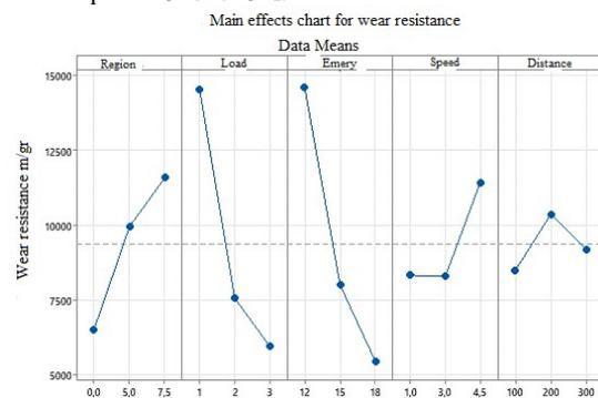
Figure 5. Key effects graphs for wear resistance
