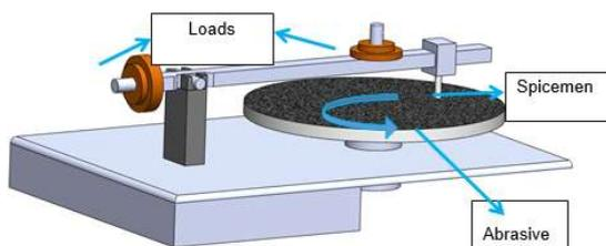
Figure 3. Schematic representation of the experimental setup
