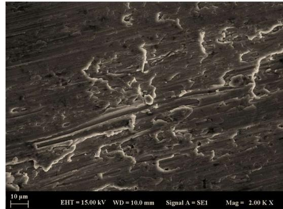
Figure 7. SEM image of the abraded surface of the not reinforced region with AIB<sub>2</sub>
