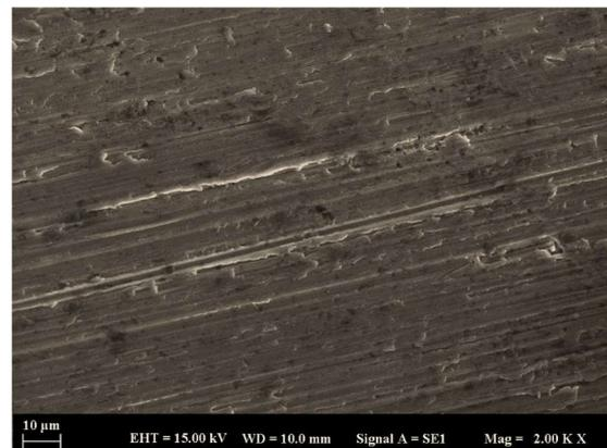
Figure 8. SEM image of the abraded surface of the reinforced region with AIB<sub>2</sub>
