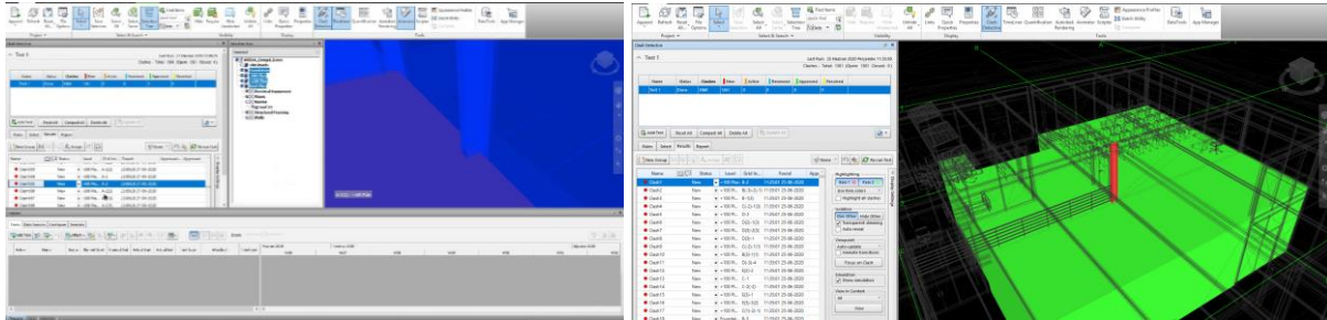
Figure 7. Transferring 3D model to Navisworks environment and defining clash tolerance rules (Drawn by Authors, 2023).
