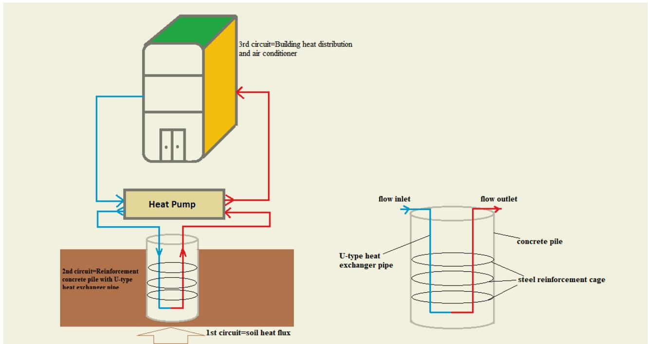
Figure 1. Energy pile cycle and its components
