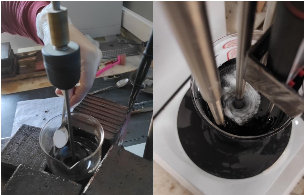
Figure 6. Production of PVC Waste-Modified Bituminous Material
