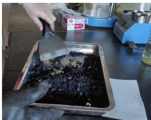
Figure 12. Loose Mixture During The Cooling Process for 2Hours
