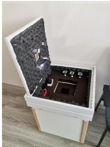
Figure 2. Specially Prepared Insulated Sound Transmission Measurement Box
