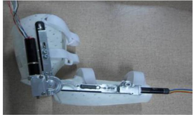
**Figure 1.** Vanderniepen home-based exoskeleton device [7].
