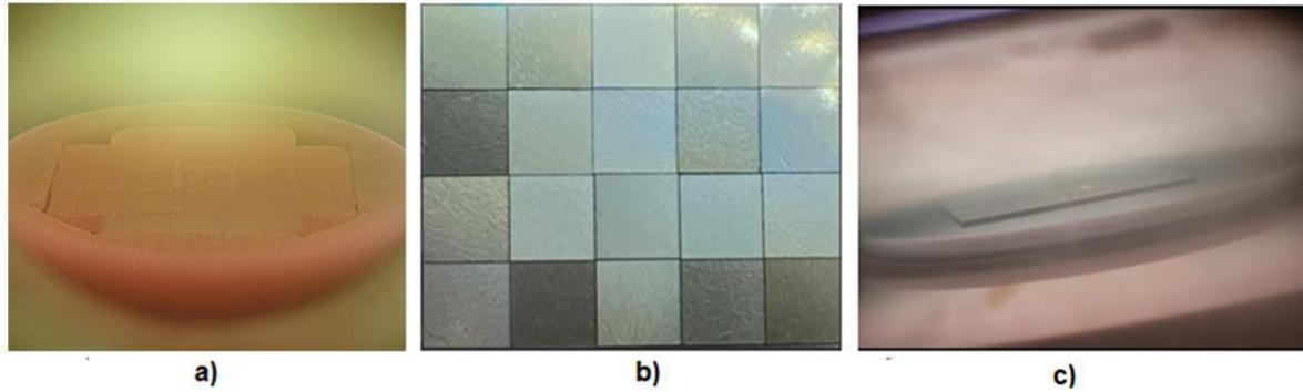
**Figure 5.** (a) Plasma formation during growth (b) Mosaic growth in reactor (c) Substrate sample
