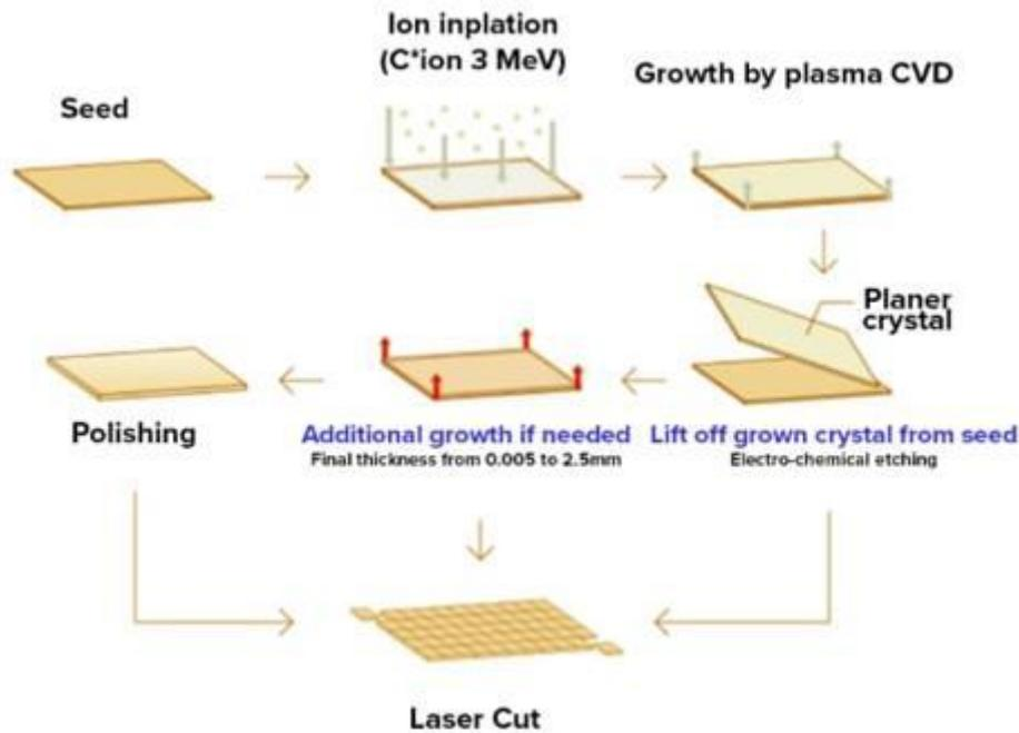
**Figure 2.** Substrate production with lift-off process
