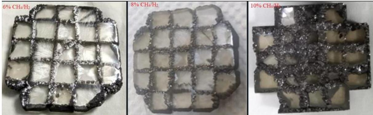
**Figure 6.** Growth result of diamond films grown with different CH<sub>4</sub>/H<sub>2</sub>ratios
