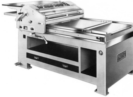
Figure 9. Korrex Frankfurt letterpress proof machines in 61x86cm. Source: (Korrex Catalogue).
