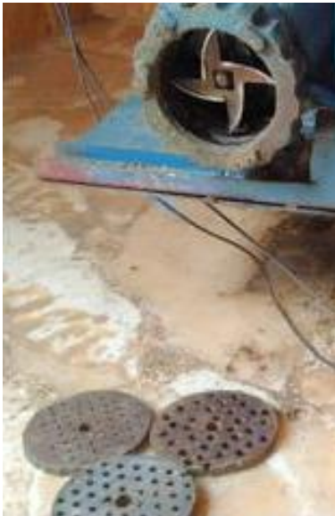
Figure 1. The machine used for pelletizing poultry litter.
