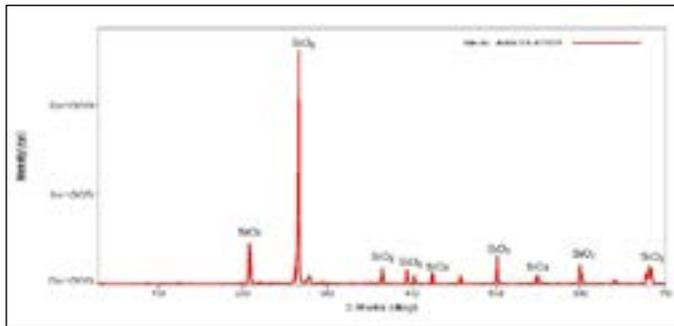
Figure 2. XRD pattern of the tailings sample
