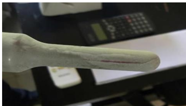
Figure 2. Core surface cracks
