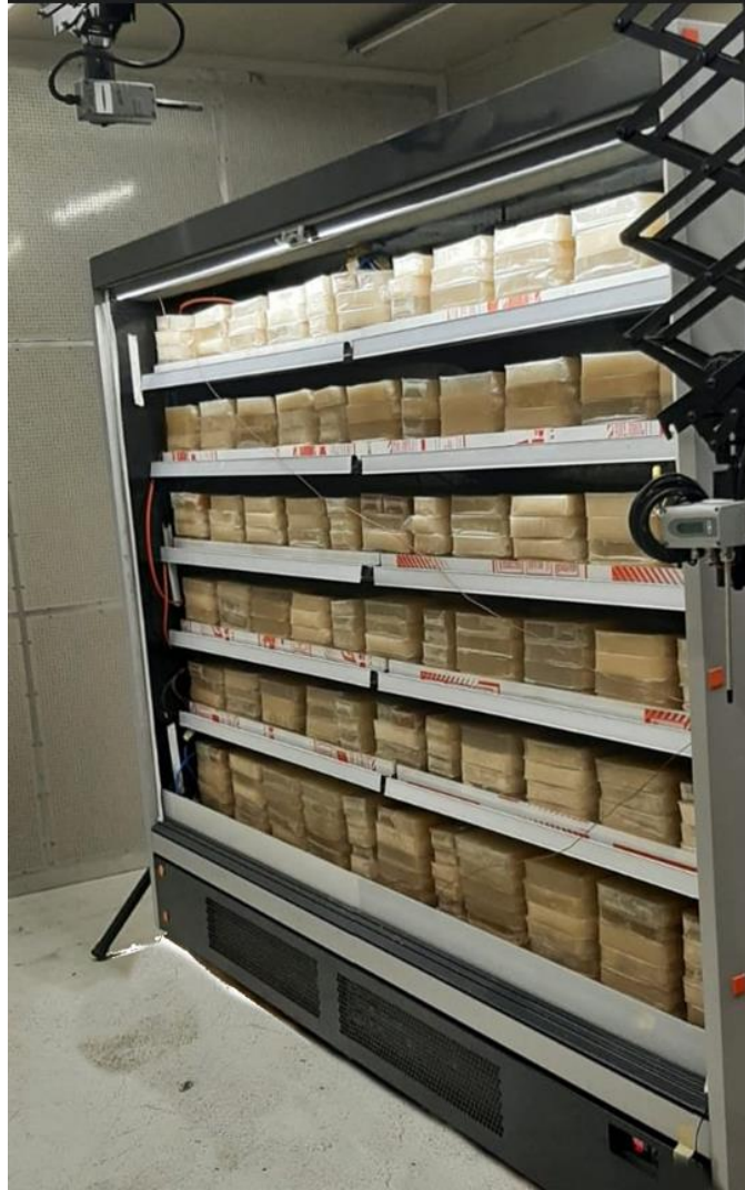
Figure 3. Photograph of the tested refrigerated display cabinet
