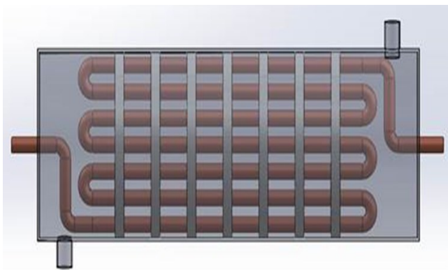
Figure 13 Designed heat exchanger with the placement of optimum number of plates, i.e. 7 plates
