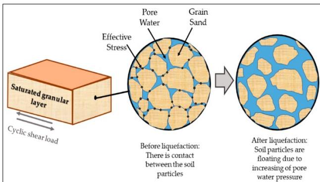
Figure 1 Liquefaction mechanism: soil particles floating due to the increment of pore water pressure [1]
