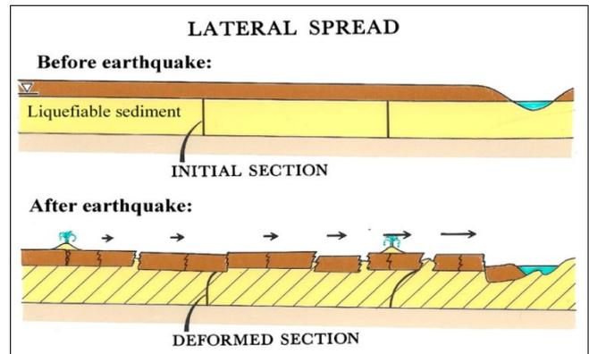
Figure 2 Schematic representation of lateral spreading [1, 3]
