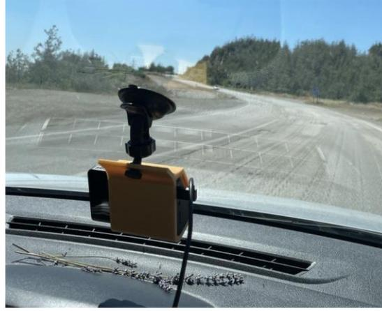
**Figure 5.** 70mai Dash Cam 4K A800S and vehicle integration
