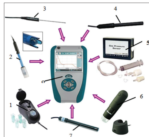
Figure 4: Modern digital laboratory, (1) Sensor of optical density colorimeter/Col-Bta (colorimeter); (2) pH sensor/Ph-Bta sensor; (3) temperature sensor/stainless steel temperature probe/Tmp-Bt sensor; (4) sound sensor Microphone/Mca-Bt (microphone); (5) illumination sensor light sensor/Ls-Bta; (6) digital wireless microscope; (7) electric conductivity sensor conductivity probe/Con-Bta; (8) processor block
