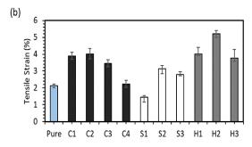
Figure 4. Tensile test results, (a) tensile strength, (b) tensile strain deviation for nanocomposites
