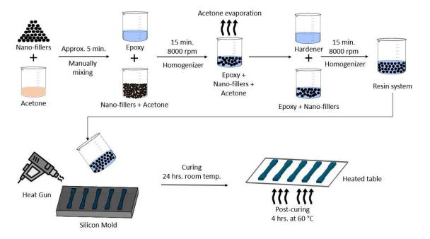
Figure 1. Nanocomposite production steps.
