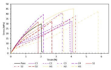
Figure 3. Engineering stress-strain curves of nanocomposites
