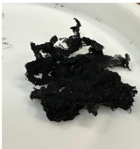
Figure 3. Sodium alginate-carbon nanotube film particles
