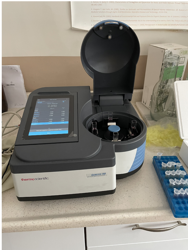
Figure 9. DPPH absorbance measurement set up for Calendula officinalis extract.
