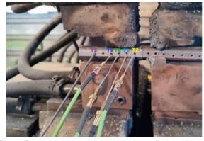
Figure 4. Arrangements of thermocouples on the sample
