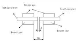
**Figure 2**. Binding of samples to the jaw
