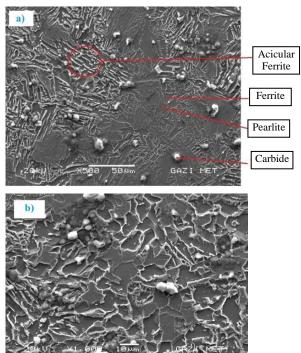
Figure 13. SEM Image of the weld metal
