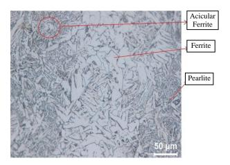
Figure 12. Image of the weld metal.
