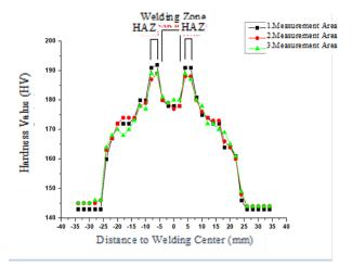
Figure 8. Graph of hardness test results
