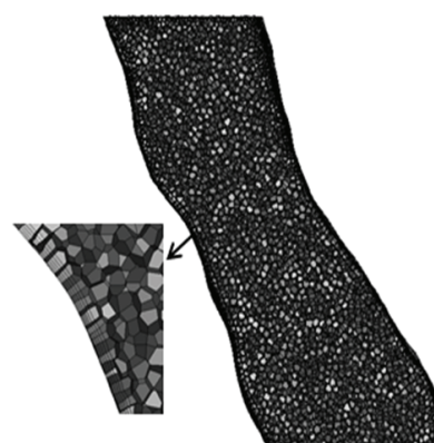
Figure 4. The polyhedral mesh and boundary layers in the trachea.
