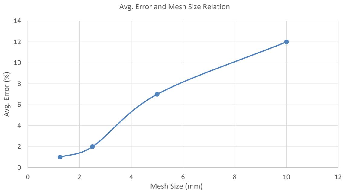
**Figure 9.** Average error calculation based on mesh size.
