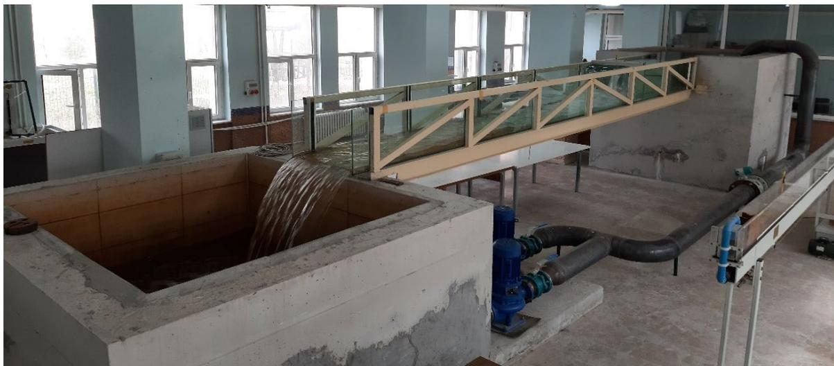
**Figure 5.** Open channel system
