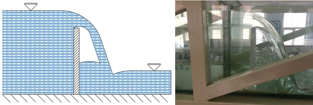
**Figure 1.** Nappe flow passing over sharp-crested weir.
