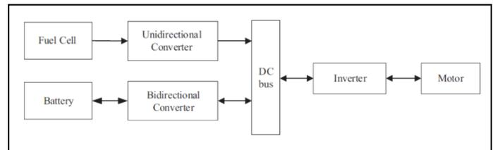
Fig. 2. Connection structure of FC - Battery HEV.
