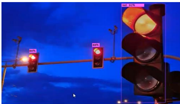
Figure 5. One result of the operation of the system. Since the work will be real-time, the FPS speed must be sufficient. In the YOLOv8 architecture, which gives the highest accuracy rate, the speed has increased to 60 FPS.
