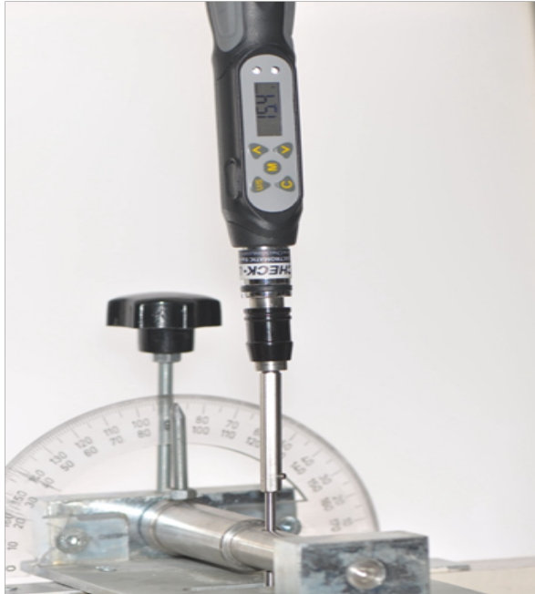
Figure 4. Maximum insertion torque measurement
