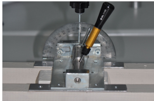
Figure 3. Mini screw application stand and angular apparatus
