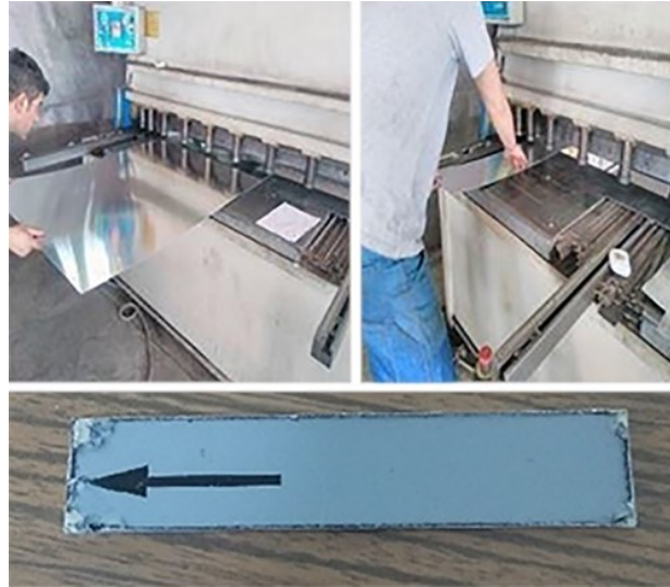
Figure 2. Cutting process of aluminum 5754-H111 adherends
