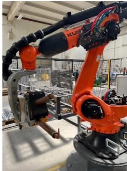
Figure 1. Robot Used In The Welding Process
