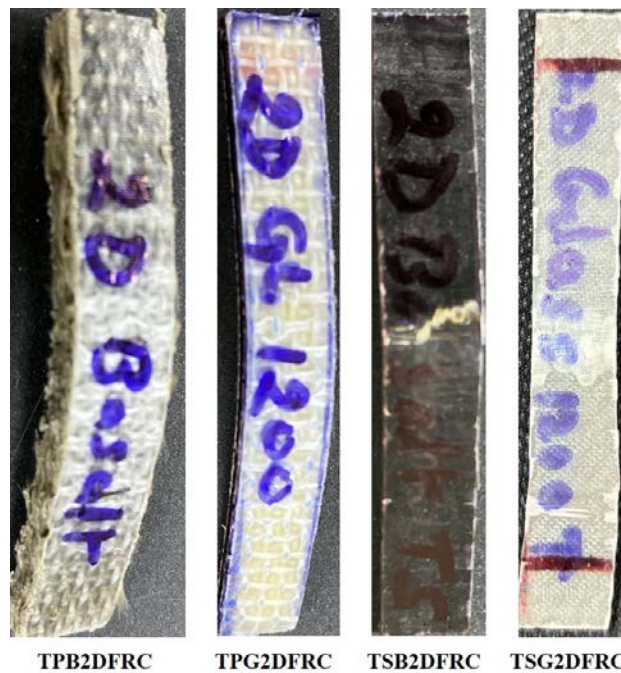
Figure 7: Flexural tested specimens at 2mm/min strain rate
