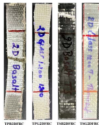
Figure 5: Tensile tested specimens at 2mm/min strain rate
