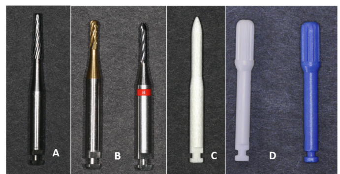
Figure 1. Four CM instruments/set of instruments A) carbide bur, B) carbide bur with titanium nitride surface treatment + fine carbide bur, C) glass fiber-reinforced composite bur, D) zirconia bur + glass fiber-reinforced composite bur.
