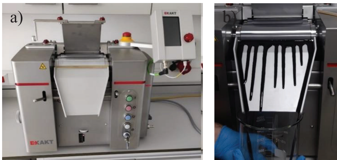
Figure 2. Three roll milling equipment (Exact 80E) and image from manufacturing.
