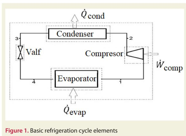
Figure 1. Basic refrigeration cycle elements
