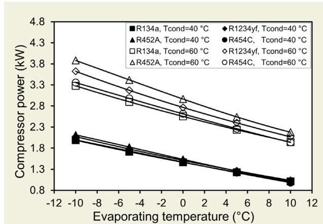
Figure 4. Variation of compressor power with evaporator temperature.
