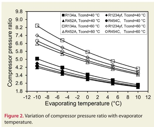
**Figure 2.** Variation of compressor pressure ratio with evaporator temperature.
