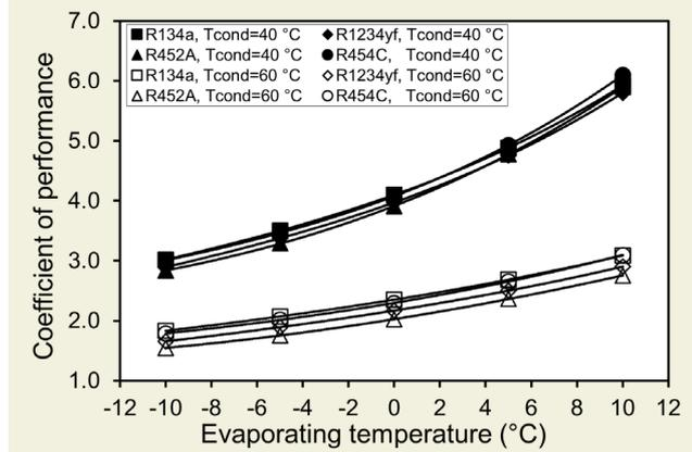
Figure 5. Variation of COP with evaporator temperature.
