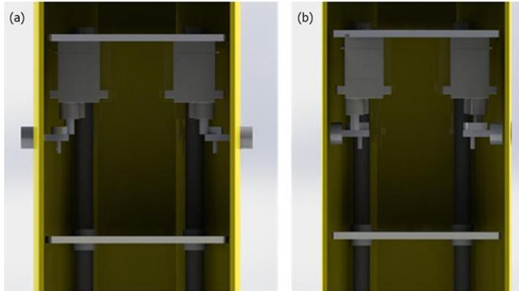
Fig. 4. Render images showing (a) the engagement and (b) the separation states of the separation mechanism.
