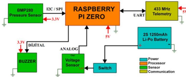
Fig. 2. Block diagram of the container system.
