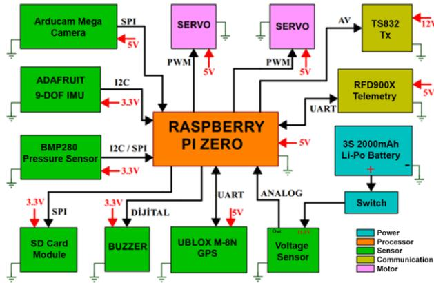
Fig. 1. Block diagram of the payload system.
