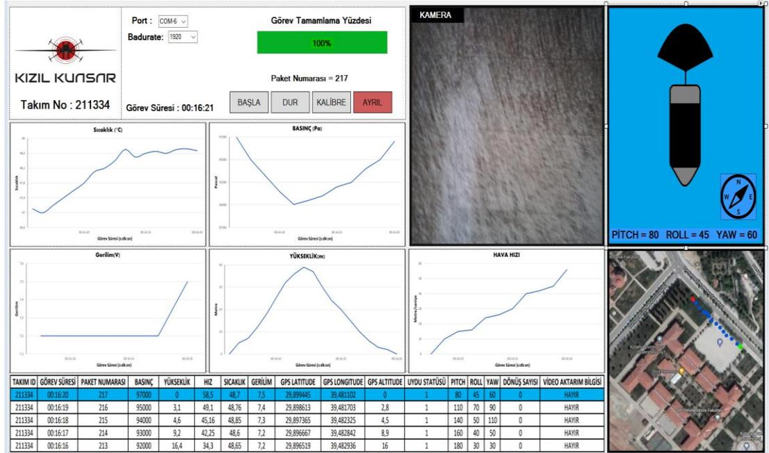
Fig. 7. The user interface of the ground station.
