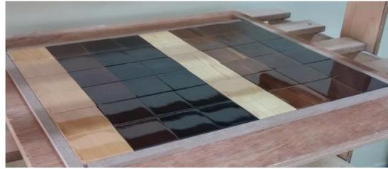
Figure 4. Drying of varnished scots pine and Eastern beech samples
