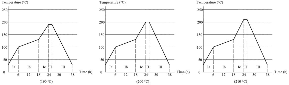
Figure 2. Heat treatment processes
