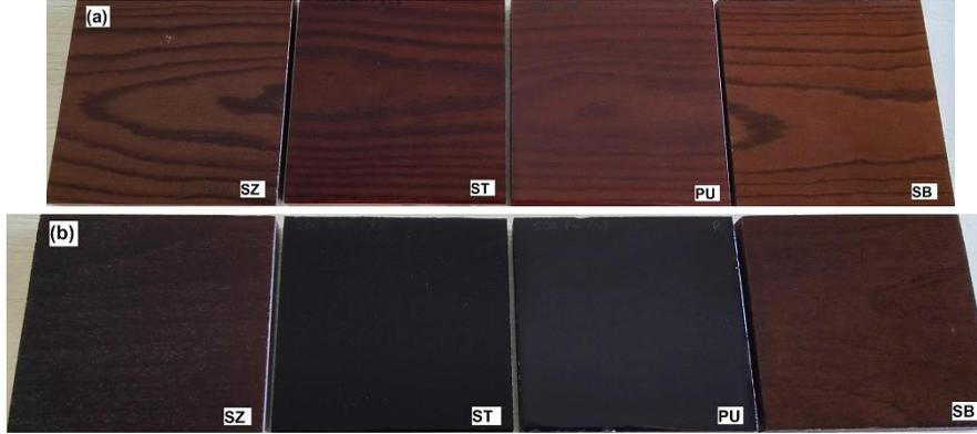
Figure 7. Appearance of scots pine (a) and Eastern beech (b) samples heat treated at 200 ° C after different varnish applications
