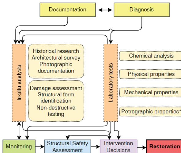
**F. 14:** Restoration steps chart of a Byzantine rock-cut structure<sup>79</sup> (Prepared by authors)
