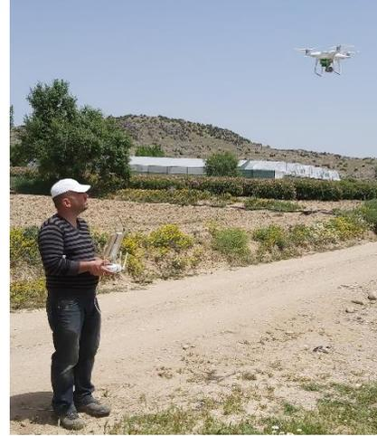
Figure 2. UAV with multispectral sensor
