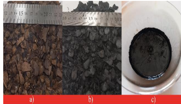
Figure 1. a) Pine cone pieces before pyrolysis, b) biochar, c) bio-oil
