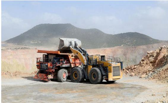
Technical Specifications of the off-highway trucks loaded by the 21 m<sup>3</sup> electric wheel loaders are as follows:
