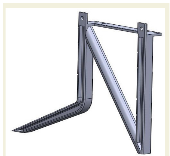
Figure 33. Improved design via topological optimization for simulation 1.
