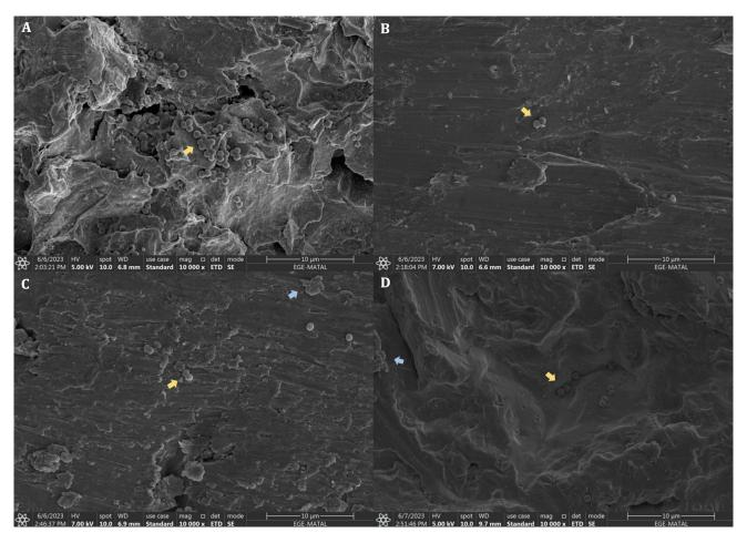
Figure 2. Representative SEM images of the S. aureus biofilm on the disc surfaces following decontamination procedures at a magnification of × 10000: (A) Control, (B) Ultrasonic-driven steel tip, (C) Ultrasonic-driven plastic tip, (D) Plastic curette. S. aureus biofilm (yellow arrow), and plastic remnants (blue arrow) remaining on the treated surfaces are indicated by arrows.
