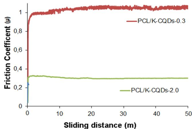
Fig. 2. Friction coefficient values of PCL/K-CQDs films.
